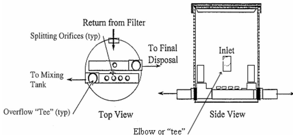
***Gravity Flow From the Recirculating/Mixing Tank Without the Use of Splitting Devices:***
