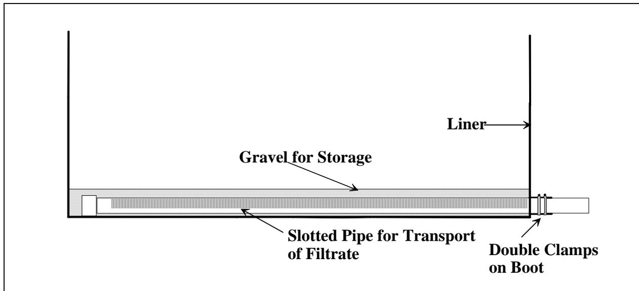
Pumpwells are located within the filter. Filtrate is collected in an underdrain system underlying the filter media and is discharged directly into the pumpwell.
